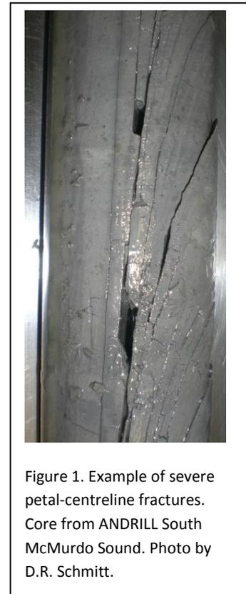
Figure 1. Example of severe petal-centreline fractures. Core from ANDRILL South McMurdo Sound. Photo by D.R. Schmitt.
