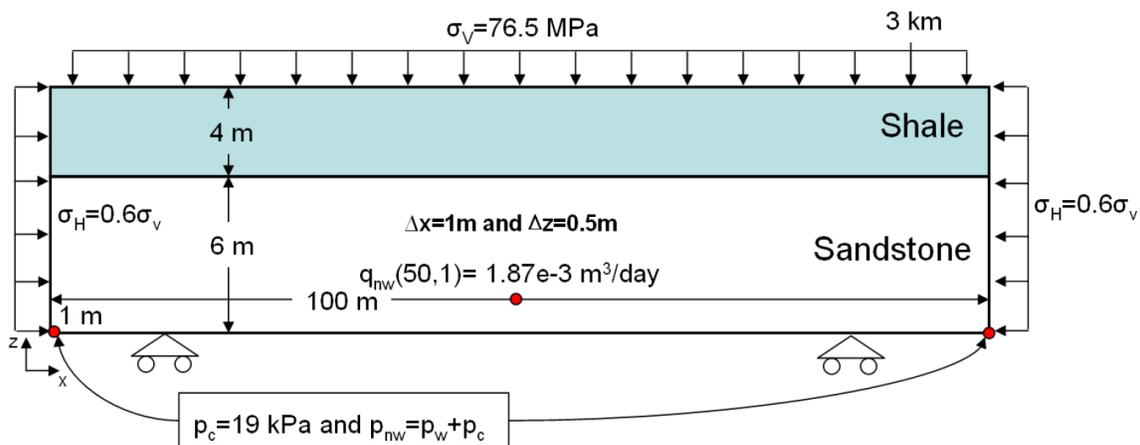
Figure 1: Model domain and boundary conditions for two-phase flow and elastic mechanical deformation for CO<sub>2</sub> benchmark
