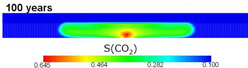
Figure 2: CO<sub>2</sub> saturation with 20 years of the injection at 100 years
