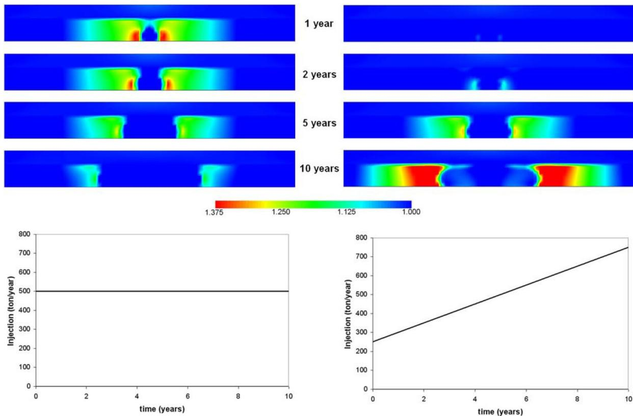
Figure 3: Safety factors for shear slip under two different injection scenarios: A uniform injection scenario in the first column and a linear injection scenario
