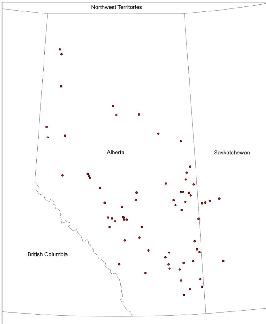
Figure 5. Location of oil and gas wells where the SCVF gas comes from the deeper production zone.
