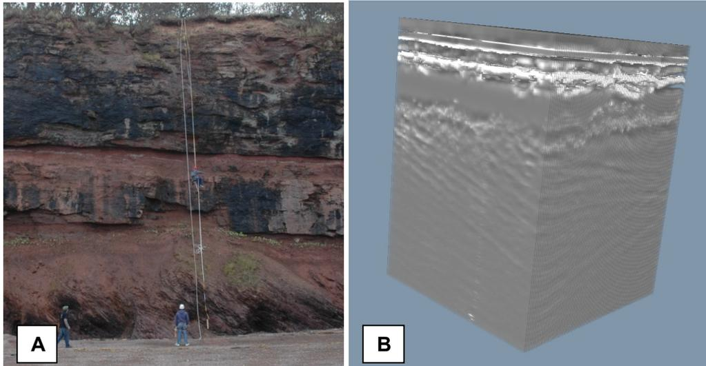
**Figure 2a:** Measuring sections, collecting scintillometer and permeameter measurements by repelling off the 20 meter cliff face. **Figure 2b:** 3D Shallow subsurface profile generated from collected GPR data.
