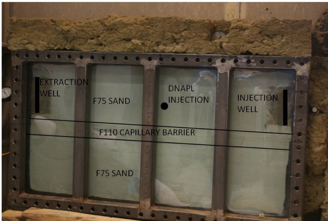
Figure 1: Laboratory cell used for steam flushing experiments
