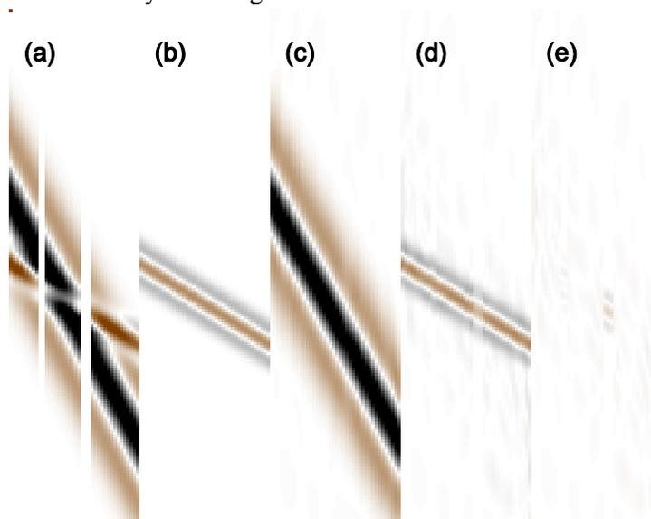
Figure 2 – Example of signal and noise separation using a synthetic primary and synthetic ground roll. The amplitude of the ground roll is twice that of the primary. (a) Input data, (b) Un-decimated synthetic primary used in (a), (c) noise model recovered by LWD, (d) clean data obtained as the interpolated difference between (a) and a decimated (c), (e) difference between (b) and (d).
