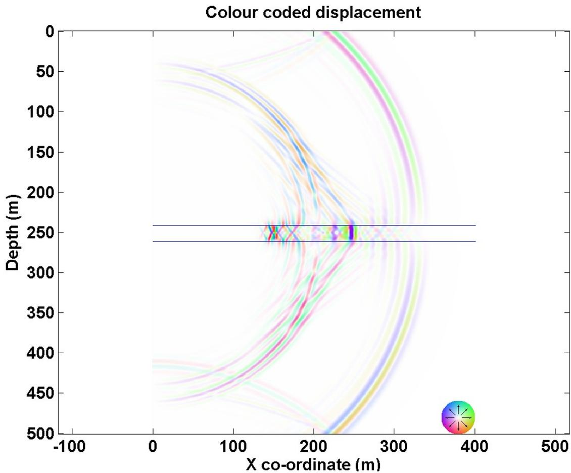
Figure 4: The wavefield model from a source at  $X = 0\text{m}$ ,  $Z = 250\text{m}$ , within a low velocity thin bed. The complexity of this wavefield would be very difficult to interpret from the limited number of geophones usually deployed.
