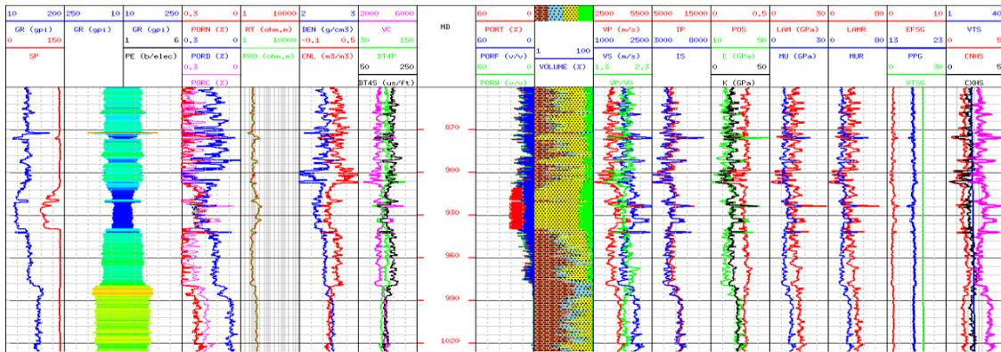
Figure 1: Well evaluation to estimate the rock mechanical property and geostress
