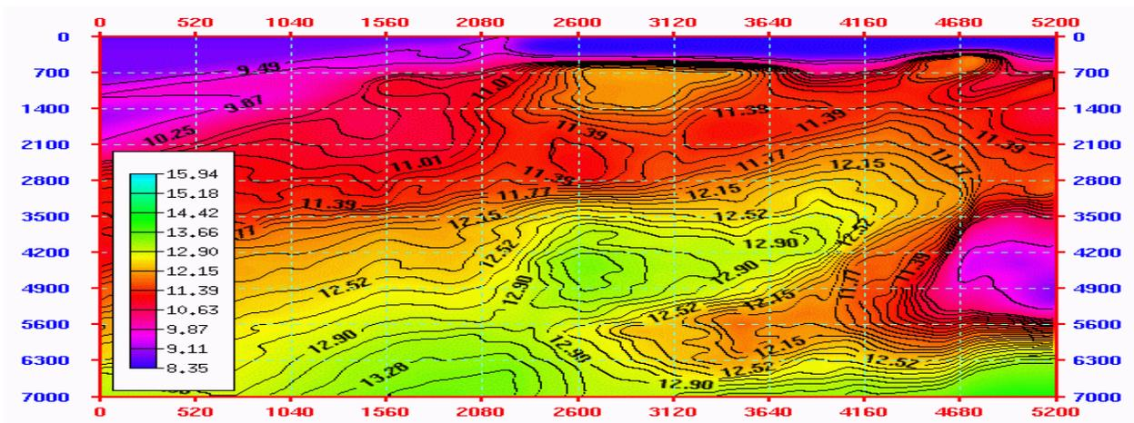
Figure 2: Pore Pressure Prediction using seismic inversion
