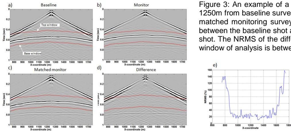
Figure 3: An example of a shot gather at x-coordinate 1250m from baseline survey (a), monitoring survey (b), matched monitoring survey (c) and the difference (d) between the baseline shot and the matched monitoring shot. The NRMS of the difference is shown in (e). The window of analysis is between the two red lines.
