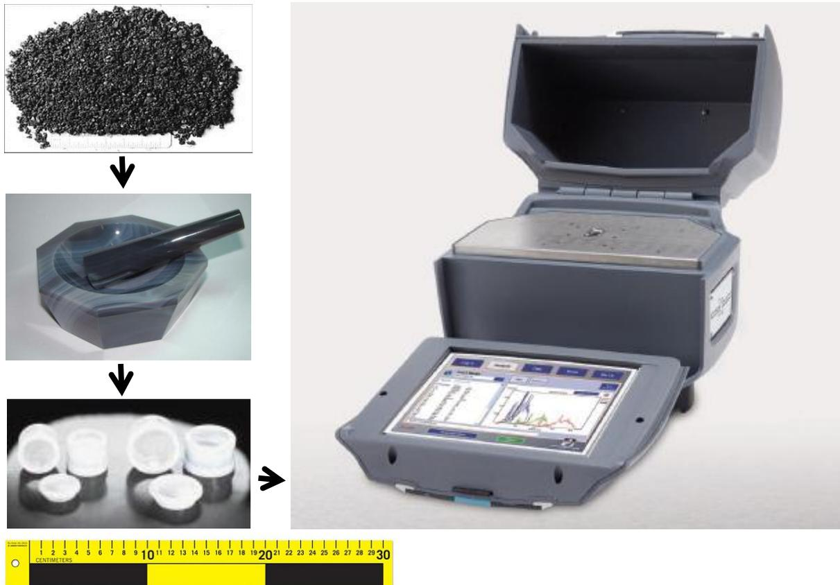
**Figure 1. XRF Analysis.** The procedure for performing XRF analysis is relatively simple. Drill cuttings are crushed in a mortar and pestle then placed into a special XRF sample cups provided by Chemplex. Each sample is run through “mining” and “soil” modes on the Innovex X-5000 portable XRF unit. It takes roughly ten minutes to crush and run a sample through both modes.
