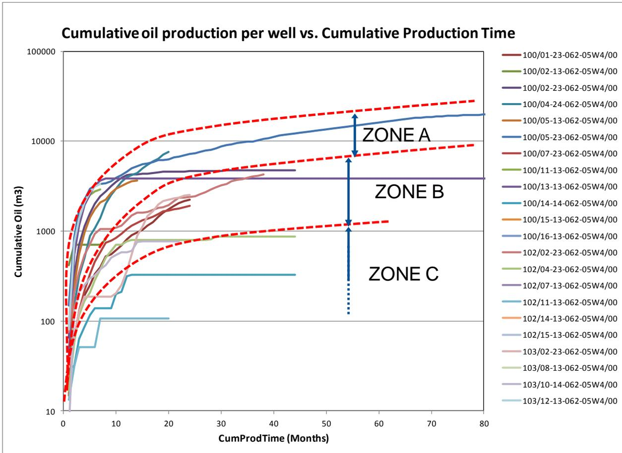
Figure 5. Cumulative oil production vs. cumulative production time for 22 wells, identifying 3 zones.
