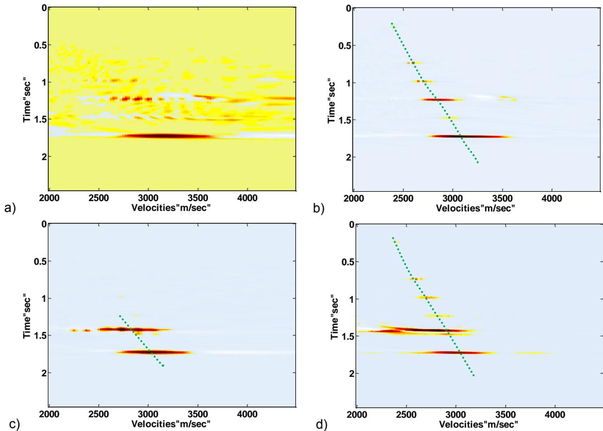
Figure 4: XC spectrum for the migration and LSPSM shot domain CIG with %10 of data. a) migration, b) LSPSM at  $x = 900\text{ m}$ , c) migration, and d) LSPSM at  $x = 2250\text{ m}$ .
