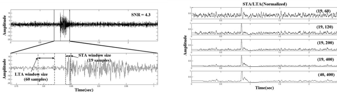
Figure 1: Left: Input microseismic data and its zoomed view. STA and LTA size are based on 2-3 periods of signal and a few periods of noise respectively. Right: Normalized STA/LTA with different window sizes.
