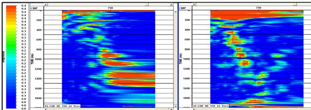
FIG. 3. Semblance display for a CMP (left) and a CSP gather (right) at the same location
