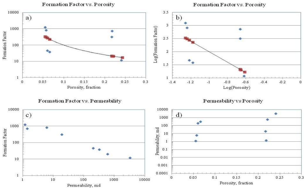
Figure 2: (a) Semi-Log plot for predicted and estimated values of formation factor vs. porosity for all cases. Solid line corresponds to Archie's Law estimation @  $m=2$  and  $a=1$ . (b) Normal scale plot for estimated values of formation factor vs. porosity. (c) Log-Log plot showing the relationship between formation factor and estimated permeability. (d) Semi-Log plot showing the relationship between predicted permeability and calculated porosity for all cases.
