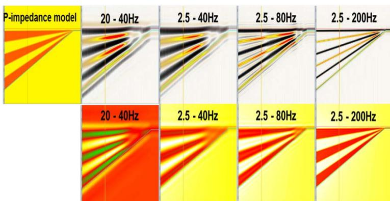
**Figure 1:** Wedge model showing seismic responses for wavelets of different bandwidth. The 4 top images illustrate the seismic responses for the various wavelets and the 4 bottom images illustrate the impedance inversions based on the modeled seismic. The color palette for the impedance sections is identical.
