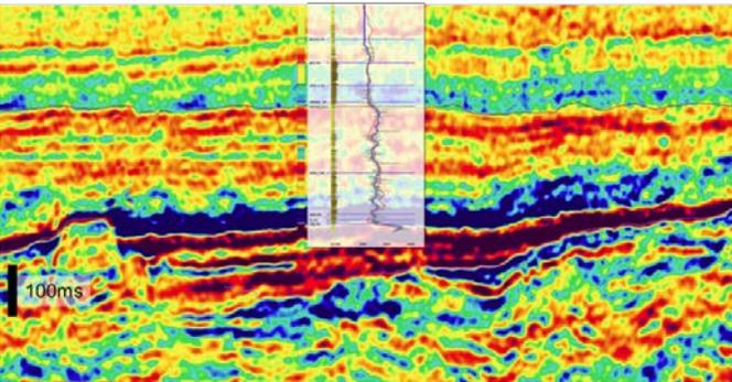
**Figure 5:** The Relative Acoustic Impedance compared to one well used as a blind well validation. Red trace is the results of the relative inversion and blue trace is the well log filtered in the seismic bandwidth.
