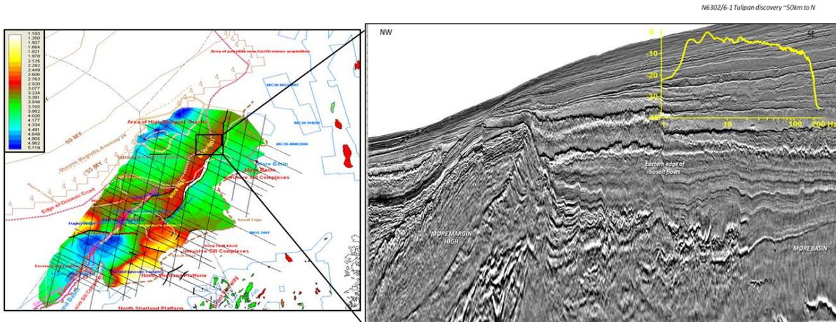
**Figure 3:** Example of a 2D seismic line over the Møre Margin High (Norway) in the Faroes Shetland Basin acquired with a ghost-free acquisition system (dual-sensor towed streamer and time & depth distributed source).
