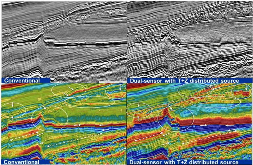
**Figure 4:** Zoom over the Møre Margin High (Norway) 2D seismic line presenting the conventional seismic response and the one acquired with a ghost-free acquisition (dual-sensor towed streamer and time & depth distributed source) system (right hand-side) and their respective relative acoustic impedance responses.
