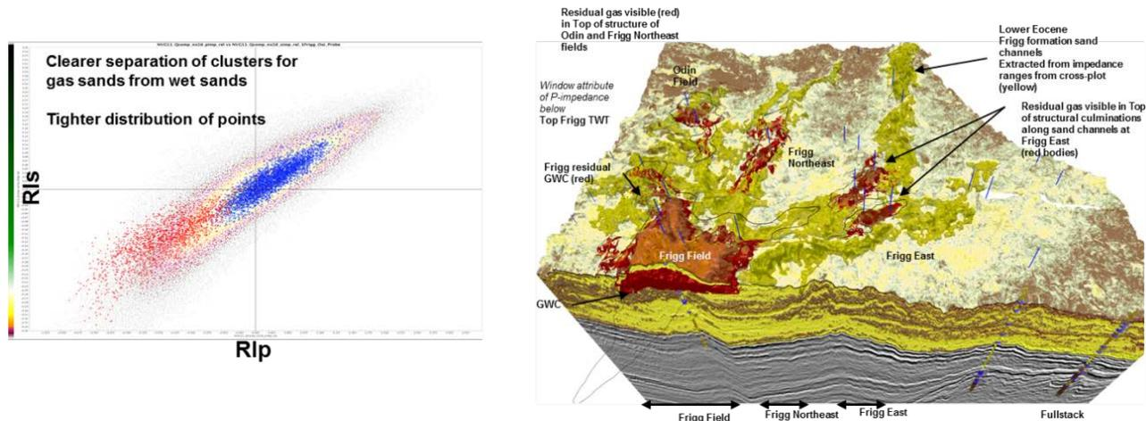
**Figure 6:** The left hand-side image represents the result of the classification in the acoustic and shear impedance domain. The blue points represent the brine sands and the red points represent the gas sand. The 3D broadband seismic was classified (right hand-side image) in term of lithology and fluid and the results are presented showing a clear delineation of the Gas Water contact as well as mapping the residual gas and channel bodies.
