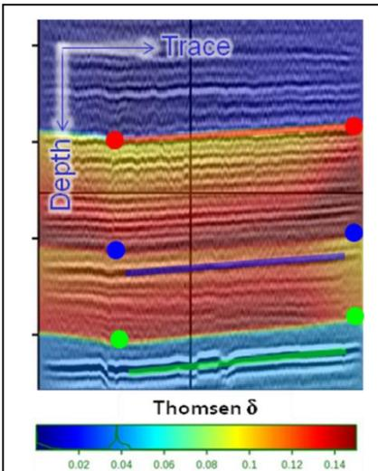
Figure 5: Thomsen  $\delta$  field overlaying seismic line. The colorbar varies from 0 to 0.15. Above the top Pierre Shale (red top), the earth is effectively isotropic. Within the Pierre Shale, we measure  $\delta$  in the 0.08 to 0.15 range. Below the top Niobrara (green top), we have no constraint on the deeper anisotropy.
