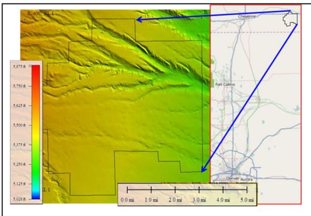
Figure 1: Burns Survey outline with topography (300 ft variation over the survey) and an inset showing the survey's location relative to Cheyenne and Denver. The receiver patch was nearly square, with a nominal fold of 150.
