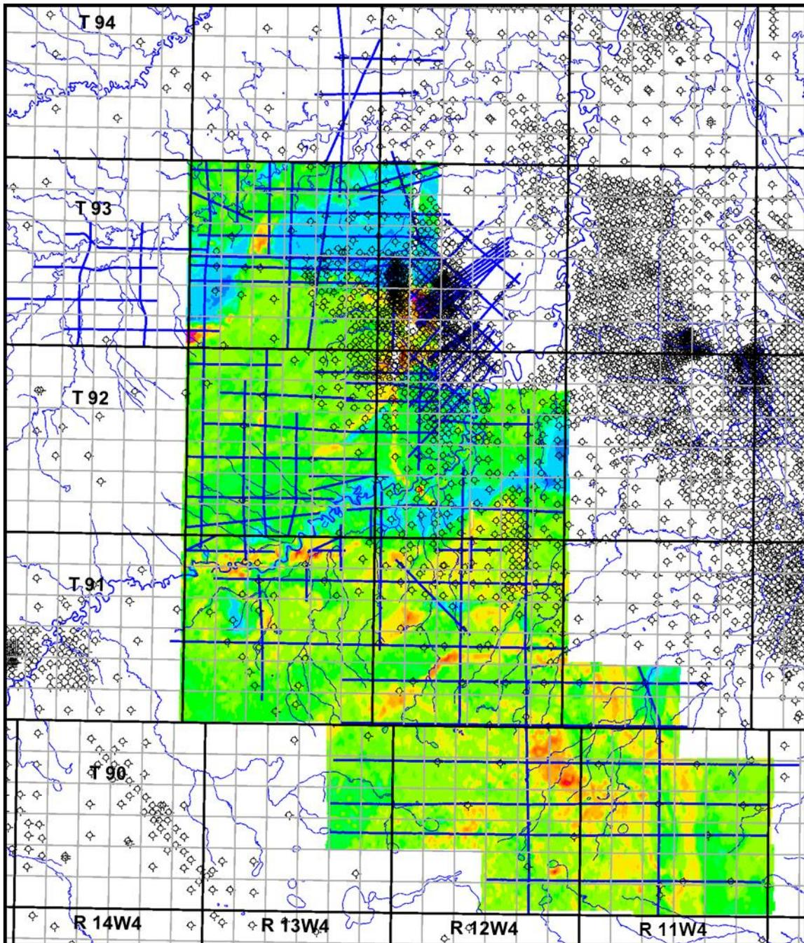
Figure 1: Corehole locations, 2D seismic database and RESOLVE aeroEM 5 metre resistivity depth slice. The single resistivity map slice alone is not diagnostic of surface material.
