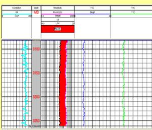
Fig.07: Computed curve for TOC based on sonic and resistivity logs using the  $\Delta\log R$  method from Murteree shale unit in Moomba-73 well.
