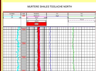
Fig.04: Computed generated curve for the TOC based on sonic and resistivity logs by the  $\Delta\log R$  method from the Murteree shale unit in Toolachee North-01 well.
