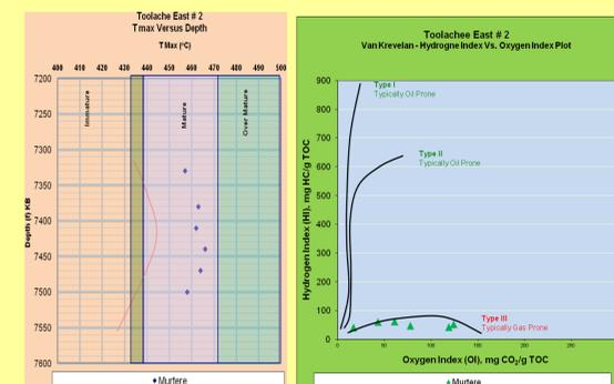
Fig.10: The Murteree shale at depth 7320 to 7550 ft is showing maturity .
