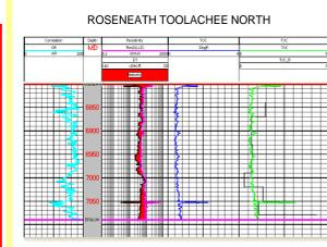
Fig.05: Computed curve for TOC based on sonic and resistivity logs using the  $\Delta\log R$  method from the Roseneath shale unit in Toolachee North-01 well.
