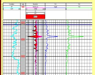
Fig.06: Computed curve for TOC based on sonic and resistivity logs using the  $\Delta\log R$  method from Murteree shale unit in Murteree-02 well.
