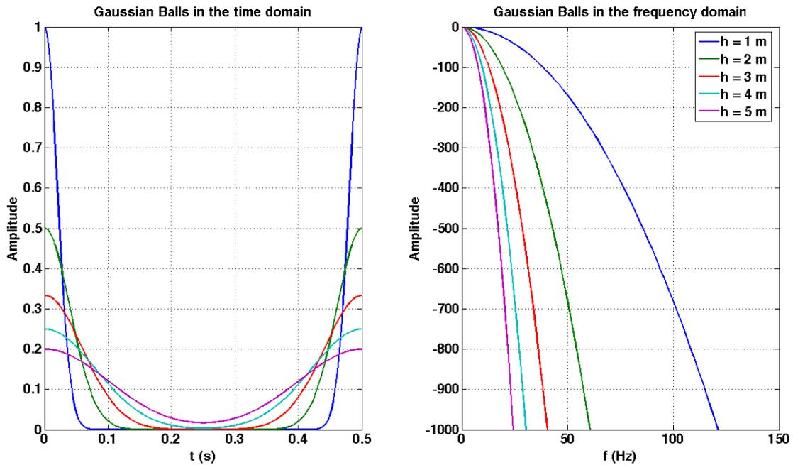
**Fig. 3.** A series of GBFs with varying ball width. Note that as the width of the Gaussian balls decrease in the time domain, their respective frequency spectra broaden. We observed a similar effect with cavity radius in the SHCM.
