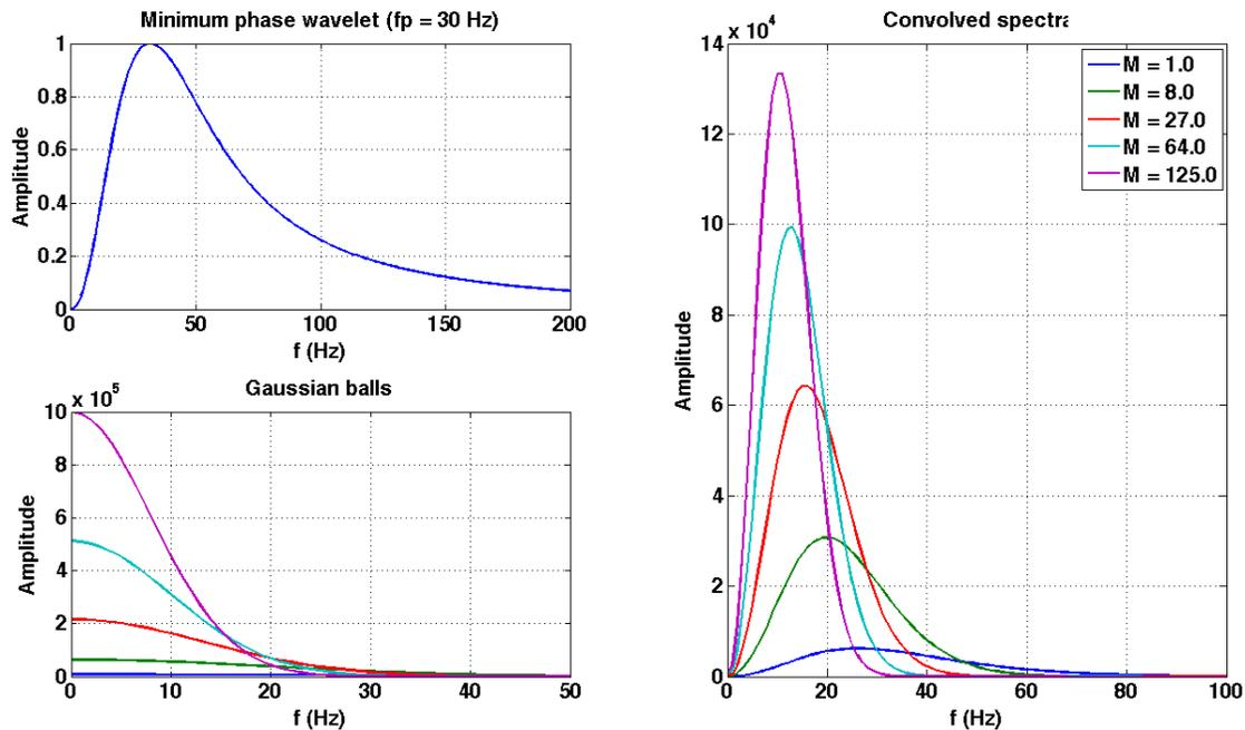
**Fig. 5.** A minimum phase wavelet that has been convolved with a series of GBFs of varying ball width. This frequency spectra that results from this wavelet also fulfils the criterion that was established in a previous study involving the SHCM.
