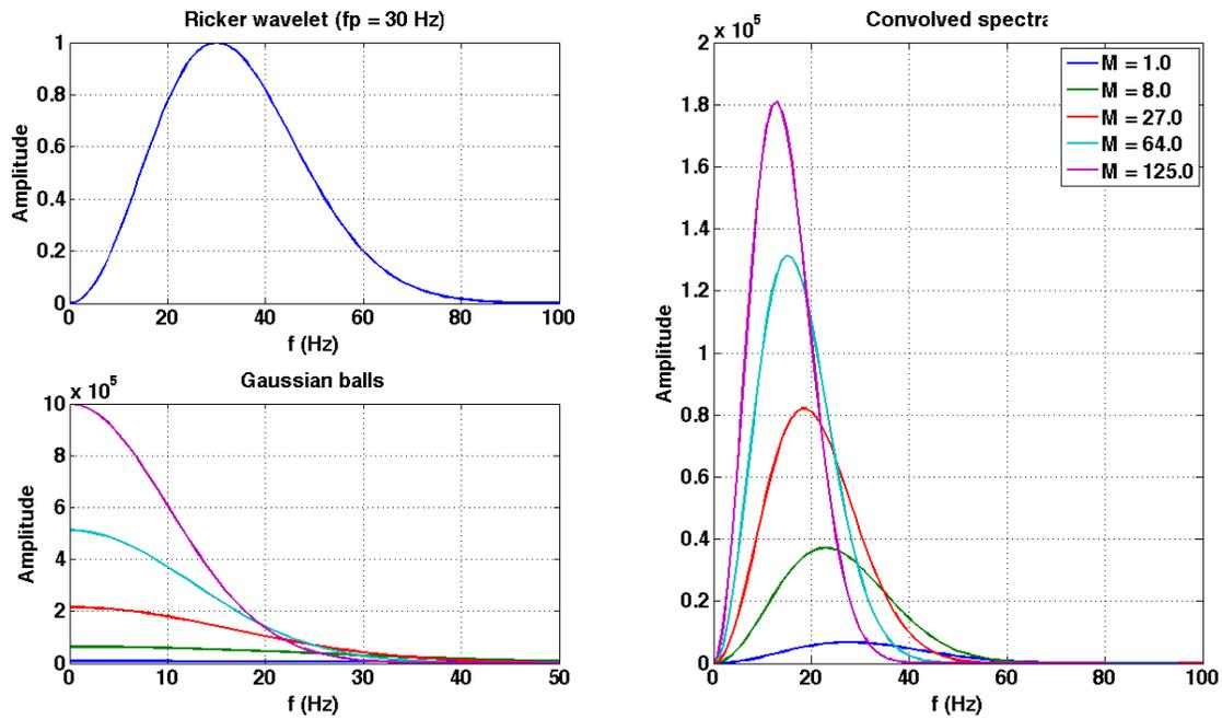
**Fig. 4.** A Ricker wavelet that has been convolved with a series of GBFs with varying ball width. This wavelet produces a frequency spectra that fulfils the criterion that was established in a previous study involving the SHCM.
