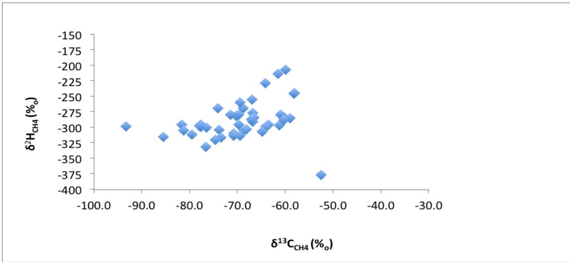
Figure 2:  $\delta^{13}\text{C}$  versus  $\delta^2\text{H}$  values of methane in free gas samples.
