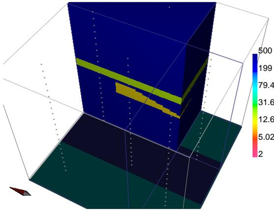
Figure 1: A sliced view of the synthetic resistivity model. The pyramid-shaped steam chamber lies below a conductive cap rock. The steam chamber and cap rock are surrounded by a uniform background. Note that the cap rock and the steam chamber are not in contact. Colourbar is in  $\Omega\text{m}$ . The gray dots show the receiver locations in the six vertical wells.
