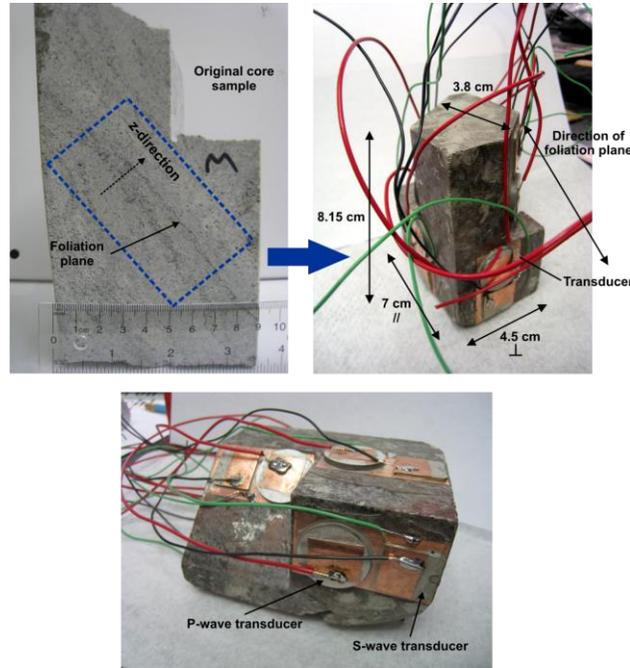
**Figure 1.** Photographs of the rock sample before (top left) and after (top right and bottom) sample preparation. Due to the limited cores available, the sample has to be carefully cut along the dotted blue lines with respect to the identifiable foliation plane in order to obtain a sample with the largest dimension possible from the core.
