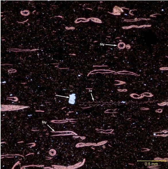
Figure 3) Plane polarized light thinsection photo of *Tentaculites* (Te) and *styliolinid* (Sty) fossils semi-aligned with bedding in an organic-rich siliceous/calcareous mudstone.
