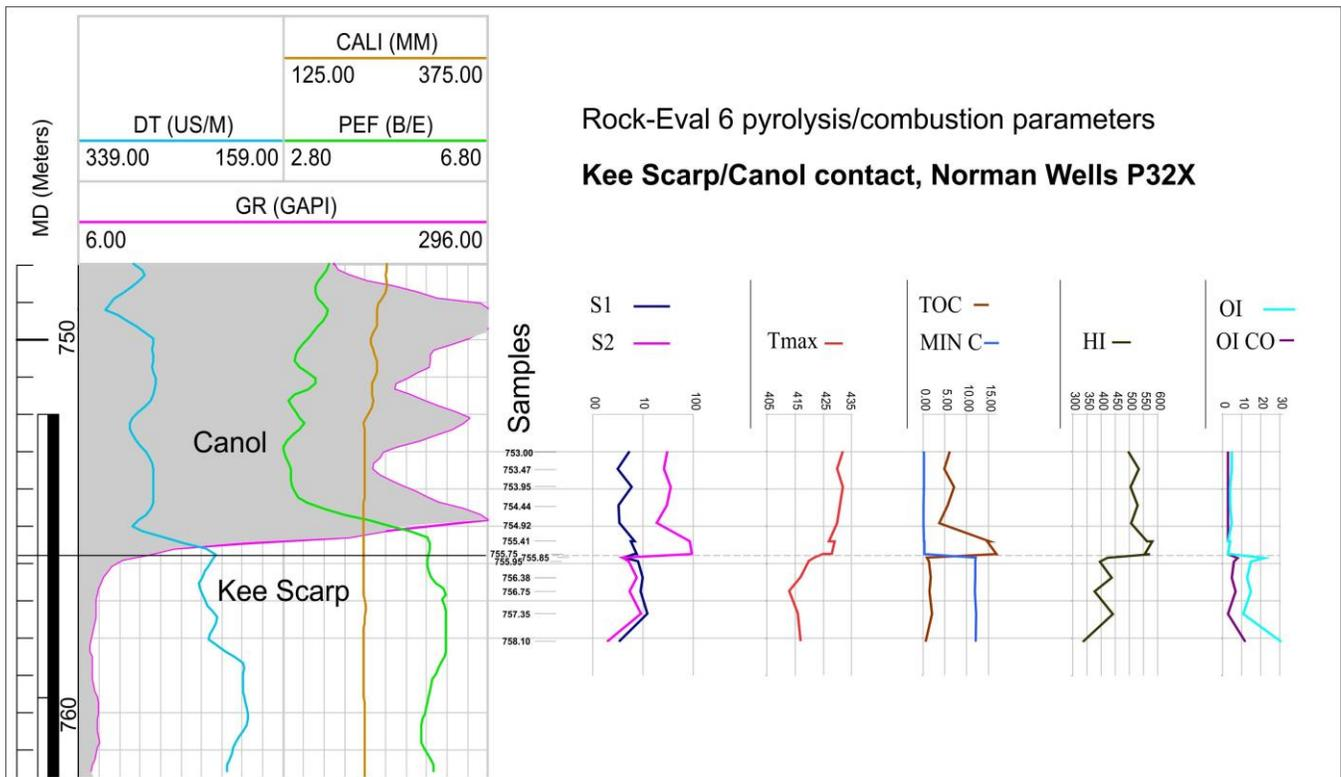
Figure 2: Norman Wells P32X: Expression of Kee Scarp / Canol contact (Fig. 1C) on borehole logs and Rock-Eval pyrolysis parameters
