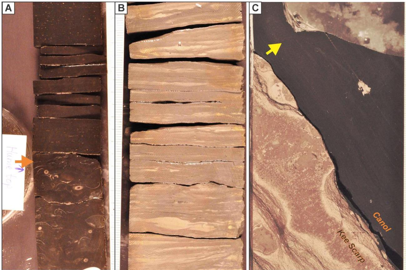
Figure 1: Shale units and their contacts with limestones: (A) Visually conformable contact of Hume limestone and Horn River black shale in Kugaluk N-02 (arrow at contact); (B) laminated calcareous shale of Headless Member (distal tempestite) deposited in lower ramp setting; (C) Kee Scarp - Canol contact in Norman Wells P32X directional well; yellow arrow shows stratigraphic up.
