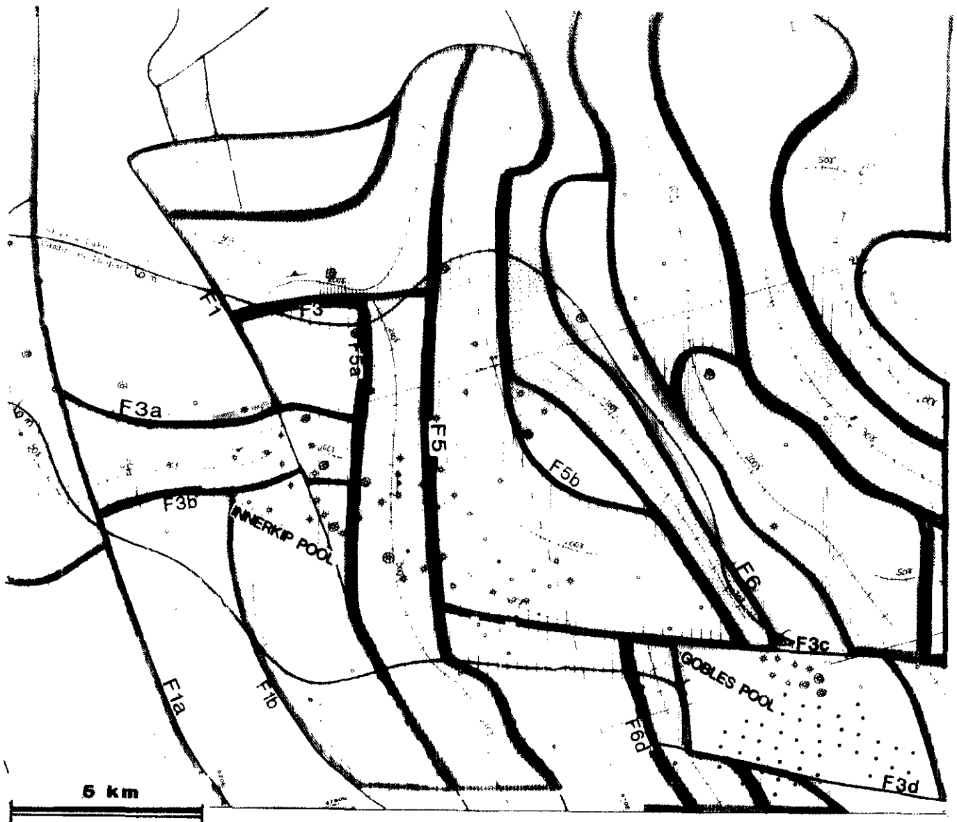
Fig. 10. Inferred Precambrian geology map including drill hole locations.
