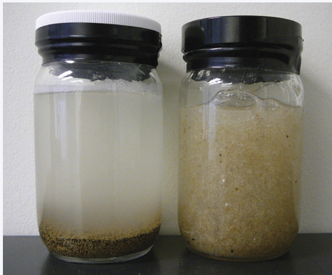
Figure 10. Several seconds after ceasing vigorous agitation the proppant is no longer suspended in slick-water (left jar) whereas the proppant remains in suspension in the gel-like consistency of the foam fluid (Schlumberger ClearFRAC base-fluid in this example; right jar).
