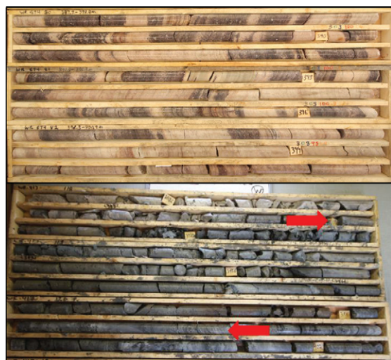
Figure 3. Photos of core of overlying sandstone (upper) and Phoenix deposit (lower between arrows) in the unconformity domain (after Reipas, 2016).
