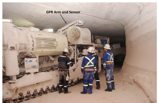
Figure 5. Picture of a mining machine (looking from front to back) at the Cory mine with the GPR sensor in the deployed position.
