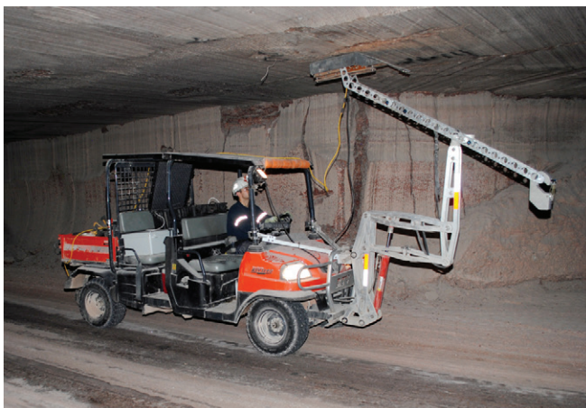
Figure 3. Kubota ATV used to collect upward-looking GPR in a typical potash mine entry.
